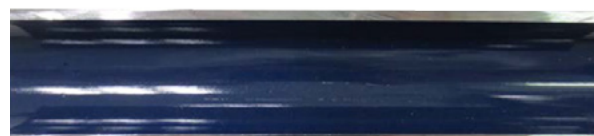
Internal finishing comparative after six months working fume condenser (non-coated and silica-based ceramic coating).
